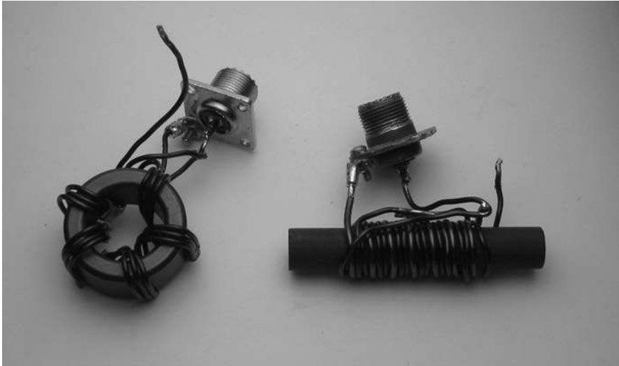
Figure 8-17 Photo shows two 1:9 ratio ununs using the schematic in Figure 8-16 to obtain operation from 1.5 to 30 MHz at the 5.56:50 \Omega level.
