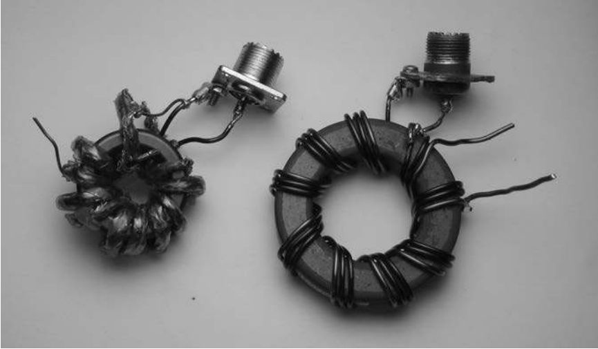
Figure 7-24 This photo shows two trifilar transformers that are tapped to give 1:2 transformation ratio.
