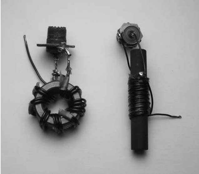
Figure 6-7 These transformers show examples of bifilar 1:4 Ruthroff transformers.
