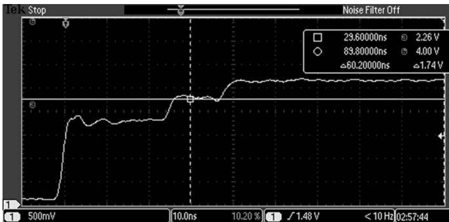
Figure 12-2 Screen capture from an oscilloscope set up as a TDR. The unknown line is a 24 in length of CAT-6 twisted pair line.
