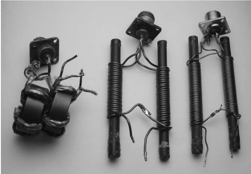
Figure 6-6 These three transformers show examples of Guanella 1:4 unun transformers.
